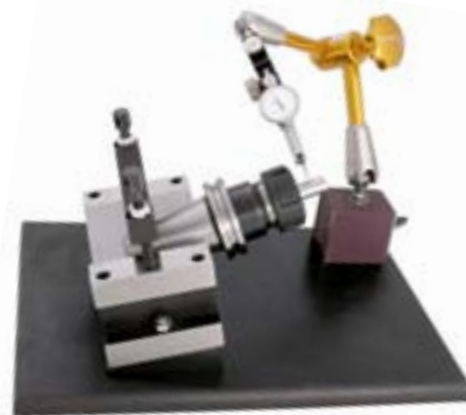
Regular bench checking of collet and nut toolholder assemblies using a gauge pin will quickly identify any T.I.R. issues.
