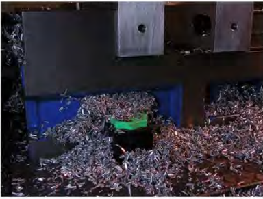
BED CLAMP SECURELY HOLDING VISE IN VERTICAL MACHINING CENTER
