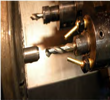
DUAL THREAD-JET ON CNC LATHE DRILLING OPERATION, WITH 32MM EXTENSION TUBES
