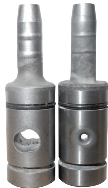
Completely worn steel mixing chamber (left) after 40 hours of use and slightly worn cemented carbide mixing chamber after 380 hours (right).
