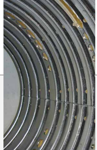
Stripping plasma layer from a jet engine casing
