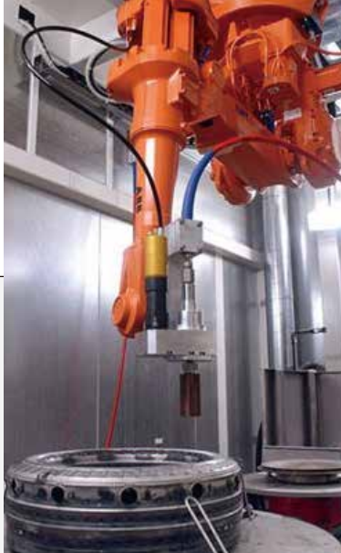
Robot with rotating head stripping plasma Coating from a cylindrical jet engine part With a turntable
