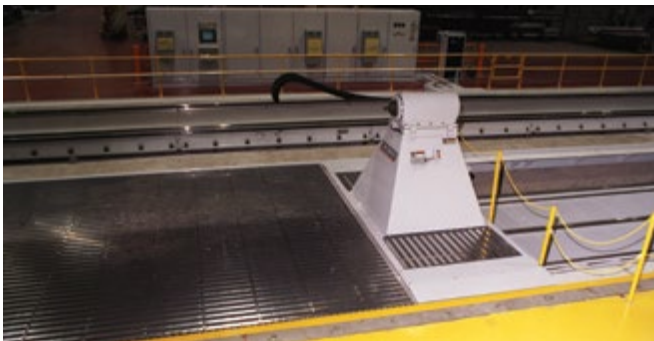
Steelflex® walk-on duty covers have been used for decades for personnel safety and machine protection, in the covering of machine ways and inspection pits.
