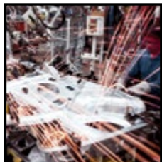
Bellows Exposed to Weld Splatter
