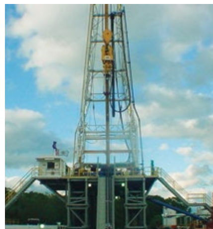
Custom 91-foot long Gortrac stainless steel LRC carrier maintains cables and hoses on an oil rig platform. Dynatect supplies many custom engineered carrier systems to the oil and gas industry.
