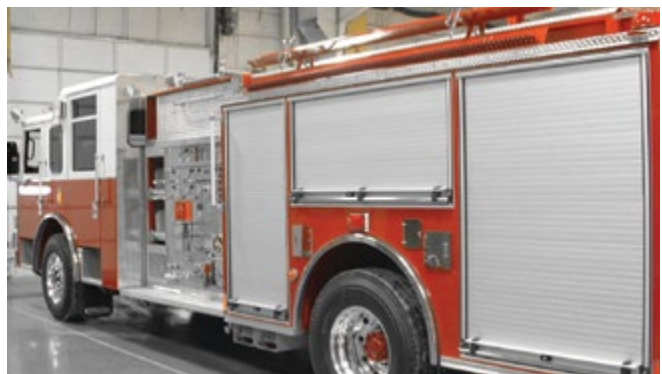
Gortite® aluminum roll-up doors are used on fire and emergency vehicles, work/utility trucks, and other commercial vehicles.
