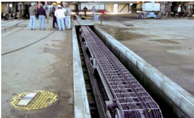
Custom stainless steel Gortrac® LRC carrier system with rolling carriage for a rocket launch system in California. Driven end modified for customer's application requirements.
