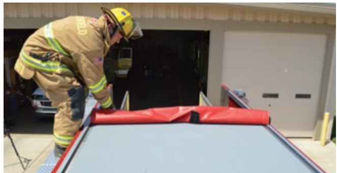
Heavy-duty roll-ups can be applied to fire truck hose beds as a retractable cover, and a walk-on surface when not in use.
