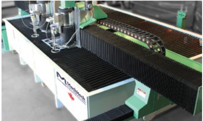
Gortite bellows and Nylatrac ® cable carriers on a waterjet machine.
