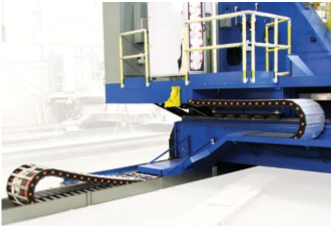
Nylatrac Modular TL carriers designed for long travel on a multi-axis riveting machine. The open-style carrier (lower left) is equipped with aluminum flat bars and low-friction modular sliders in a lowered mounting height configuration. The enclosed-style carrier (upper right) shields cables from ejected rivet heads and debris with heavy-duty bolt-in aluminum armor plates.
