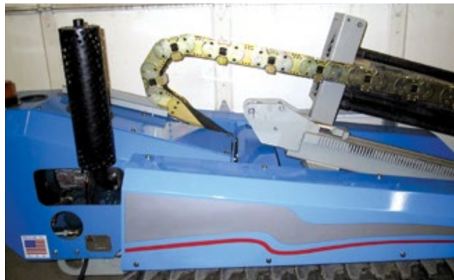
Gortrac steel SRC carrier with window extenders on underground boring equipment.
