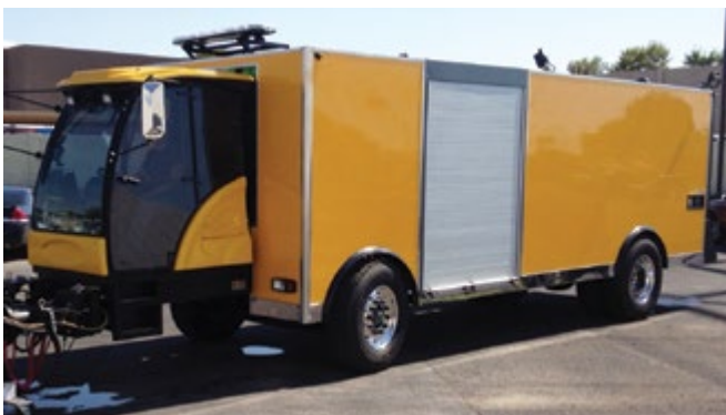
Gortite® aluminum roll-up doors are used on fire and emergency vehicles, work/utility trucks, and other commercial vehicles.
