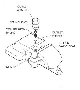
12. Clean and inspect the check valve body and outlet adapter.
