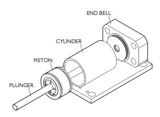
Remove the cap screw(s) holding the remaining end bell to the assembly fixture and set aside.
