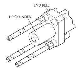
12. Install the filler tube in the high-pressure cylinder.
