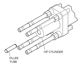
51. Reinstall the check valve assembly and end cap by sliding it along the tie rods and guiding the high-pressure cylinder into the bronze bushing of the end cap. Take care to align the check valve assembly with the correct orientation as previously noted in Step 5.
