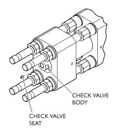
6. Using fresh solvent, clean the threads and bore of the outlet adapter and check valve body.
