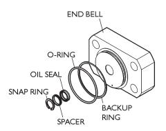
19. Clean the hydraulic cylinder, end bells, oil seal spacers and snap rings. All service must be completed in a clean, well-lit area.
