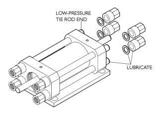
39. Draw the low-pressure cylinder carefully onto the end bells by tightening the nuts evenly in a figure-8 pattern, as shown below. Be careful not to nick the seals and back-up rings. There must be no seal or back-up ring debris visible at the cylinder/end bell interface. Be sure to check for any problems before continuing. Following the figure-8 pattern shown below, torque all nuts evenly to 20 ft-lb (27 N-m) to seat all parts.
