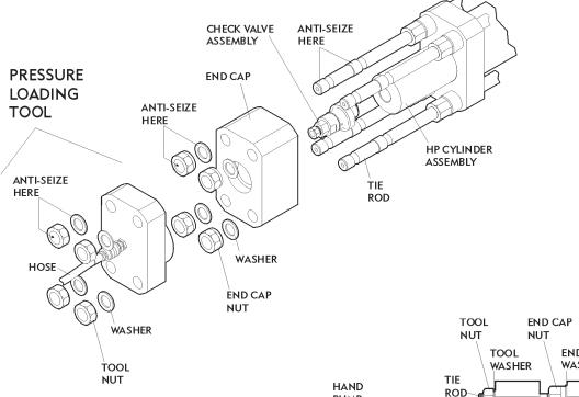
The illustrations on this page identify the parts used in this procedure, and provide a visual description of how the tool assembles to the tie rods of the intensifier.
