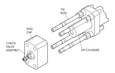
7. Remove the high-pressure cylinder and filler tube from the intensifier end bell. Rocking the cylinder gently while pulling outward is helpful in separating the cylinder from the end bell. When the cylinder is clear of the end bell pull it straight out to avoid the ceramic plunger.
