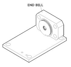
35. Apply clean hydraulic oil or Parker Super O-Ring Lube to both plungers. Install the cylinder by inserting the plunger into the end bell.
