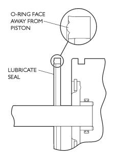
30. Slide the piston and plunger assembly containing one seal into the cylinder so that the empty groove enters the cylinder first. Use a soft-faced mallet where necessary.
