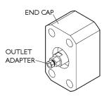
9. In a soft-jawed vise, clamp the check valve assembly on the flats machined into the body.
