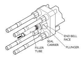
49. Install the high-pressure cylinder by sliding it over the ceramic plunger and into the end bell bushing. A slight rocking motion will help ease the cylinder into position.
