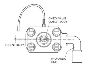
6. At one end of the intensifier, remove the end cap from the tie rods. The check valve assembly will remain in the end cap due to the compression of the o-ring on the check valve body.
