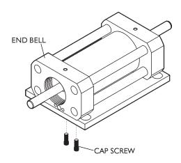
16. Remove the cylinder from the other end bell. The piston and plungers can stay with the cylinder. Do not use a screwdriver to pry the cylinder from the end bell.
