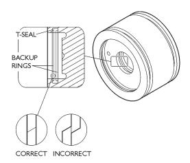
27. Apply clean hydraulic oil or Parker Super O-Ring Lube to the head of the plunger. Insert the plunger into the counter bore in the piston, using a soft mallet if needed. Make sure the T-seals do not get nicked or rolled.
