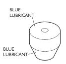
Make sure the coned end is pointing out once installed, and that there is no Blue Lubricant on the sealing face of the outlet check valve seat.
