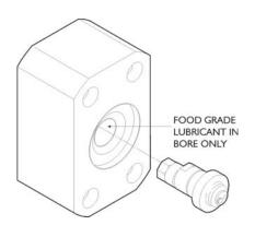
Install the new check valve assembly by pushing it into the end cap. Take care to align the check valve assembly with the correct orientation as previously noted in Step 6.
