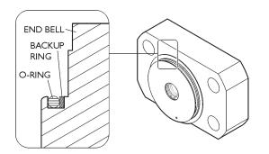
Reinstall the o-ring removed in Step 18 from the high-pressure cylinder side of the end bell.
