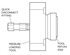
5. Connect the hand pump hose to the tool at the quick-disconnect fitting (see below).
