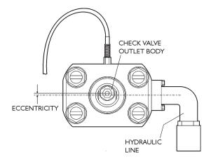
6. Remove the end cap from the tie rods. The check valve assembly will remain inside the end cap due to compression of the o-ring on the check valve body.
