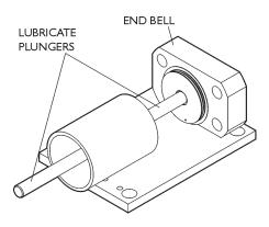
36. Slide the remaining end bell over the other plunger and seat it on the assembly fixture.
