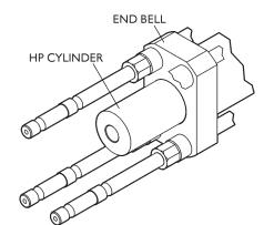
50. Install the filler tube in the high-pressure cylinder.
