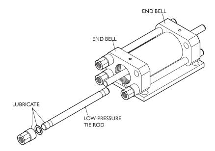
38. Apply anti-seize lubricant to the exposed threads of the tie rods and the faces of the washers and nuts. Install the nuts onto the tie rods hand tight.
