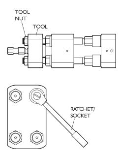
10. Using the ratchet and socket, back off the tool nuts **exactly one** full turn.
