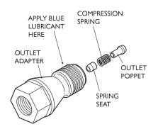
10. Thread the outlet adapter into the check valve body. Torque to 200 ft-lb (271.2 N-m).
