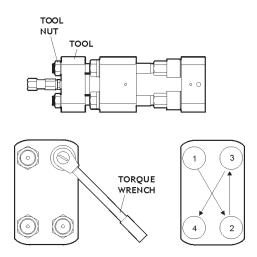
9. Pump the tool to 9200 psi (634 bar).
