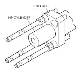
10. Reinstall the filler tube in the new high-pressure cylinder.
