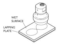
15. Turn the lapping plate over and place a few drops of water on the 600 grit side of the plate. Lap the check valve body in a figure-8 pattern until the body is evenly polished.
