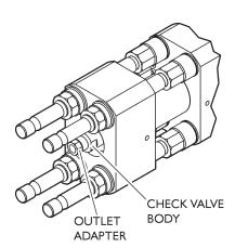
4. Remove the outlet poppet, compression spring, and outlet spring seat from the outlet adapter. Discard the poppet and spring, but set the spring seat aside.
