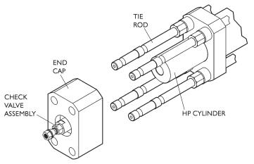
7. Remove the high-pressure cylinder and filler tube from the intensifier end bell. Rocking the cylinder gently while pulling will help separate the cylinder from the end bell.
