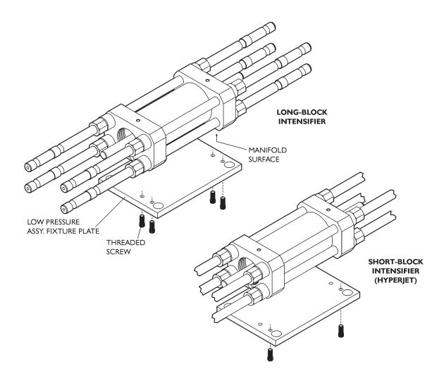
13. Remove the high-pressure tie rods.
