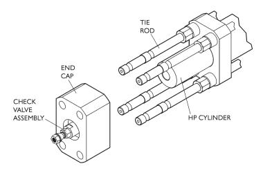
8. Remove the check valve assembly from the end cap by pushing on the outlet adapter (see illustration at right). Set the end cap aside.
