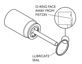
33. Slide the piston and plunger back into the cylinder. Take care when the seal is being compressed as it enters the cylinder—the seal can easily be damaged by rough handling at this point.
