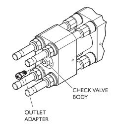
9. Apply Blue Lubricant to the surfaces of the new outlet check valve seat as shown and insert it into the bore of the check valve body.
