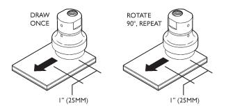
17. Carefully clean the newly-lapped check valve body with clean solvent such as isopropyl alcohol. Dry and re-inspect the part.
