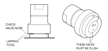
14. Attach a 320 grit abrasive strip to one side of the glass plate, and a 600 grit strip to the other side.
