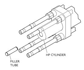
11. Thoroughly clean the tie rods, nuts, and washers to remove the old anti-seize lubricant.
