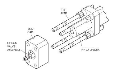
8. Remove the old check valve assembly from the end cap by pushing on the outlet adapter (see illustration below).
