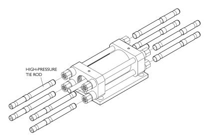
14. Use the ratchet handle and torque multiplier (as shown here) to loosen the tie rod nuts at **one** end of the low-pressure cylinder assembly.
