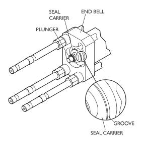
11. Slide the high-pressure cylinder over the ceramic plunger and into the end bell bushing. A slight rock-ing motion will help ease the cylinder into position.
