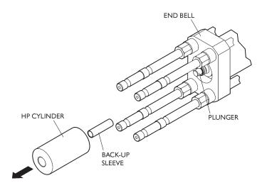
8. Pry the seal carrier away from the end bell using a small pry bar in the groove provided, as shown.
