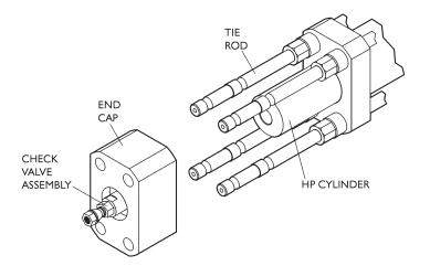
7. Remove the high-pressure cylinder and filler tube from the intensifier end bell. Rocking the cylinder gently while pulling will help separate the cylinder from the end bell.
