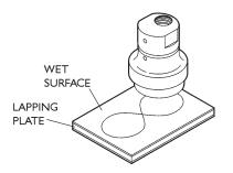
16. To avoid poppet sticking problems, turn the lapping plate back to the 320 grit side and draw the check valve body for 1 in. (25 mm) in a straight line along the abrasive strip once, then rotate the body 90° and repeat the 1 in. (25 mm) score.
