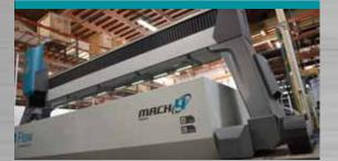
With durable design throughout, the Mach 4 is made up of precision machined and thermally stress-relieved solid steel castings, easily handling even the most rigorous use day in and day out.
