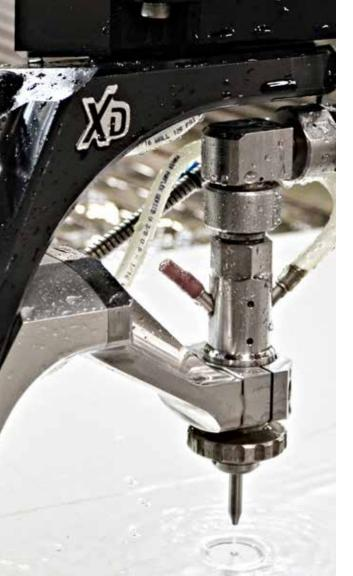
(+/- 0.03 to 0.08mm). The technology allows the machine to move very fast, create a taper and stream lag, and then compensate for it automatically by tilting the head by up to 10 degrees.
