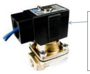
Typical solenoid. This model <u>is part number A-</u> 12812 which is popular with most Flow pumps. Always check to see if components like solenoids are bi-directional installing a replacement unit. This model is not and has an "in" port and an "out" port. If solenoid is not working, check for control voltage at din connector. Most modern pumps are 24VDC while older models are 110 VAC.
