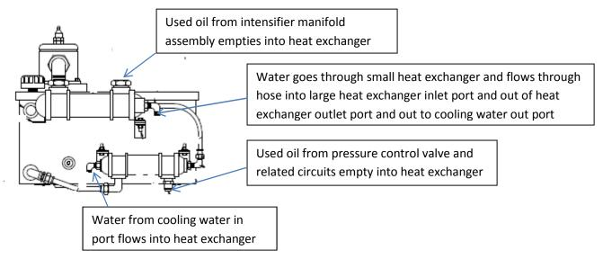
Dual heat exchanger setup as found on 5X, 7X, 9X and 50i.s. intensifier pumps.
