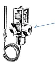
Cooling water control valve; part number A-6851. Turn adjustment screw clockwise to allow more water to go through cooling system. Remember this is a mechanical device so give the system 30-45 minutes to regulate and stabilize. Another part of the cooling system is the solenoid. Most systems have the same solenoid on the filtered water in port that is on the cooling water in port. Make sure that the solenoid is opening and allowing water to pass.
