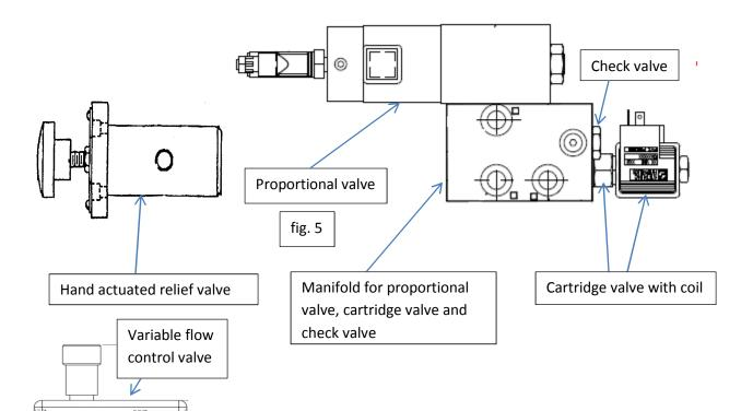
The other parts of the hydraulic system include the reservoir that holds the oil for the hydraulic pump fig. 1-2-3, to use and return to, manifolds fig. 5 and hoses for transmitting hydraulic fluid from component to component in the hydraulic system.
