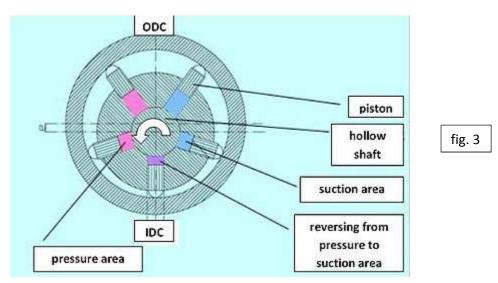
Here is a basic example of the radial piston pump;
