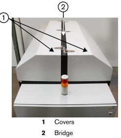
1. Remove the screws at both ends of the bridge. If there are not screws in the location shown, remove the outermost hinge screws.
