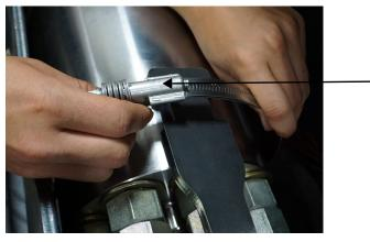
3. Put the guard straps over the tabs on the top of the attenuator guard.
