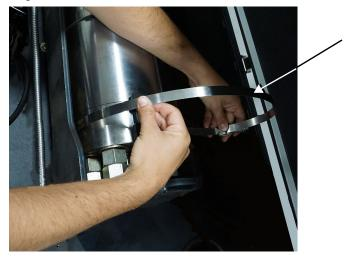
2. Put the ends of the guard straps into the bolt drives.
