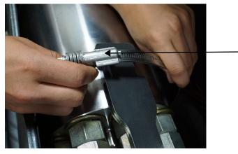
3. Put the guard straps over the tabs on the top of the attenuator guard.
