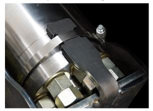
4. Turn the bolt drives clockwise to tighten the guard straps.
