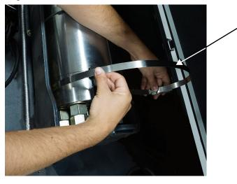
2. Put the ends of the guard straps into the bolt drives.
