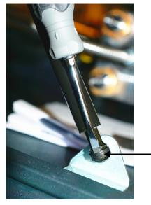
b. Hit the shock with an open hand to release it from the ball.
