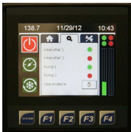
Figure 2. This screen is used to enable/disable the intensifier(s) and pump(s) and adjust the overstroke percentage. Red represents disabled and green represents enabled.
