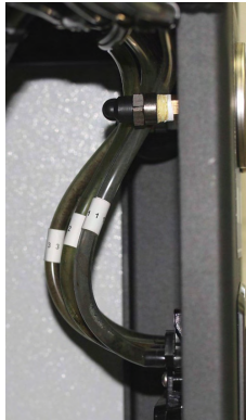
Good tube routing
