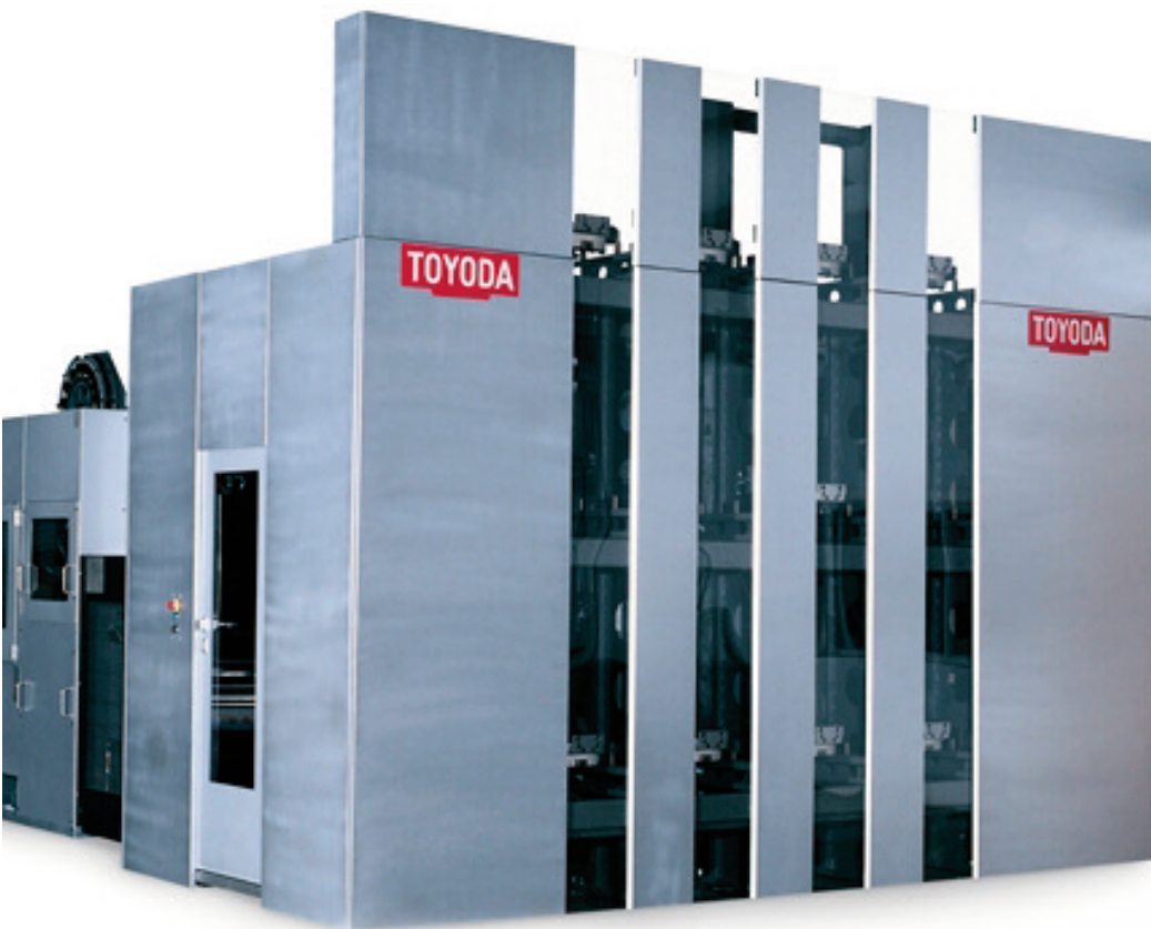
NEW 2013! Toyota FH800SX-i with 800mm x 800mm pallet, envelope 59" x 59"h, 308 Tools, 20 Pallet pool
