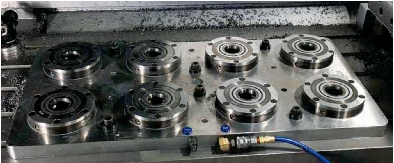
The ERGO E800 preassembled bases shown with custom mounting holes to match the T-slot pattern of the customer's machine.
