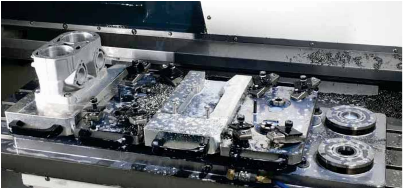
The ERGO E1000 preassembled base shown with four customer-designed fixtures. Standard fixture pallets are available in either aluminum or steel and various sizes and thickness. Please see UNILOCK Vol. 2, Pg. 70-71.
