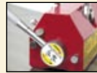
Lever in the "ON" position. The safety lock is engaged.
