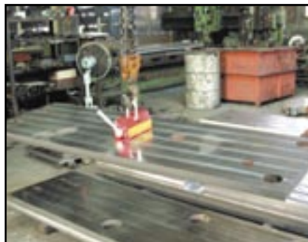
Locate magnet at balance point for lifting.
