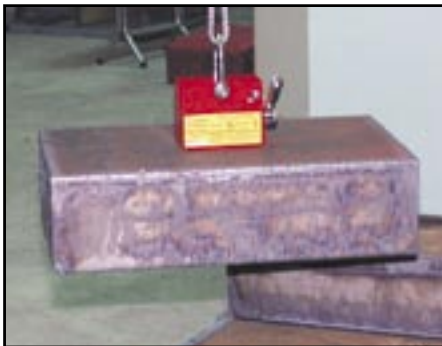
Center magnet on workpiece to lift.
