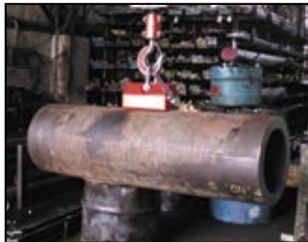
Beveled bottom surface lifts tube steel easily.
