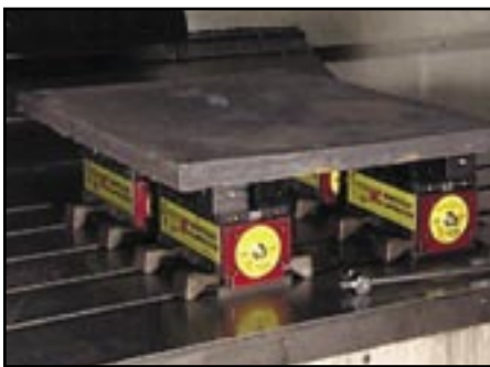
Spring-blocks adjust to hold warped stock
