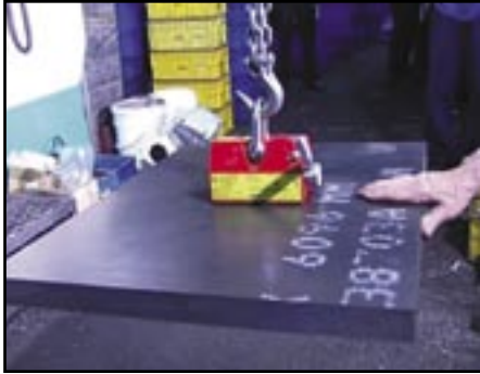
Safest way to move ferrous stock.
