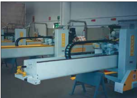
▼ P18 hand pump used for locking the rotating table for marble polishing.
