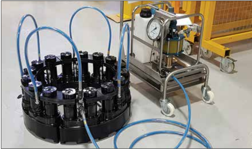
▲ Multi Stud Tensioning Set-Up.
