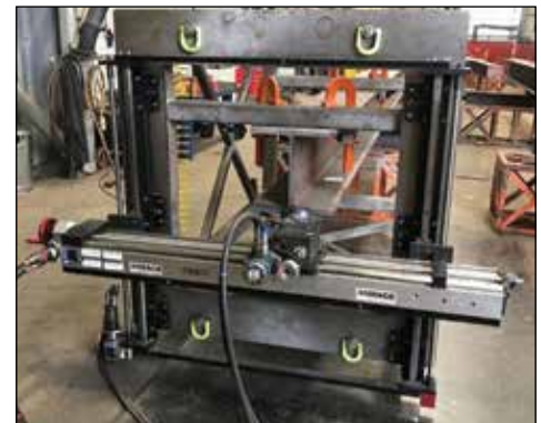
I-Beam end face milling with a GMRF1000. ▶
