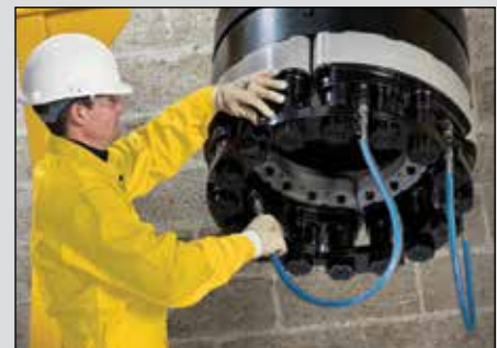
▲ Multi-Stud Tensioning application.
