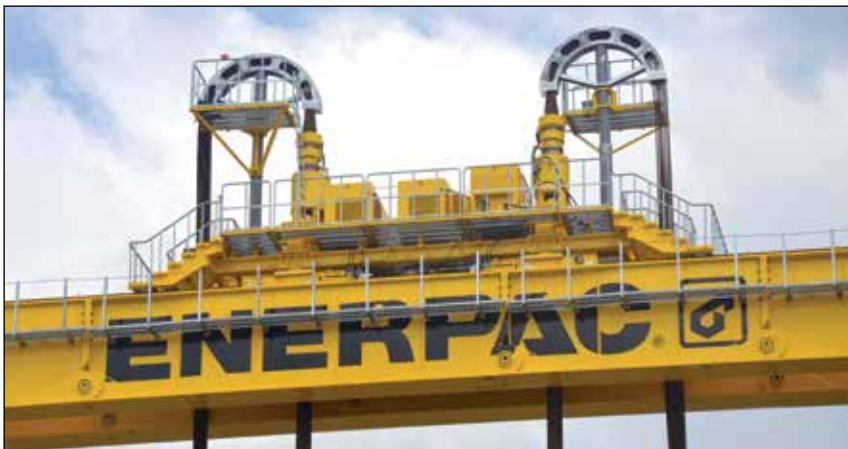
▼ Shown: HSL85007 Strand Jack System used on Enerpac custom Self-Erecting Tower.
