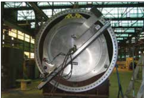
▼ Wind tower machining with WP4600.
