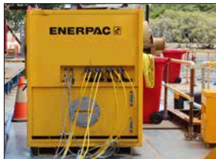
▼ SyncHoist Powerpack to operate the 4 lifting points.
