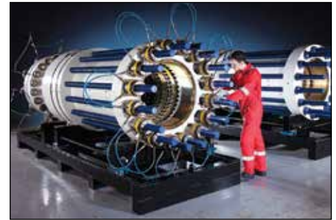
▲ Inter-connected with HT-Series hoses Enerpac subsea tensioners apply uniform bolt load.
