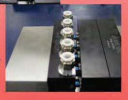
THE X-PANDER SYSTEM DRAMATICALLY INCREASES PRODUCTION OF SMALL INTERNALLY HELD PARTS, ON MANUAL OR CNC MILLING MACHINES. THE SELF CONTAINED, MODULAR SYSTEM HOLDS 5 PARTS AT A TIME ON THE ID OF EACH PART.
