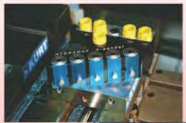
THE X-PANDER WORKS WITH THE HYDRAMAX WORKHOLDING SYSTEM TO HOLD SMALL PARTS ON THEIR ID.
