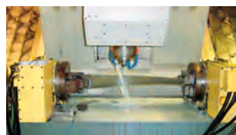
Synchronous Rotation by CNC401 X 2units
