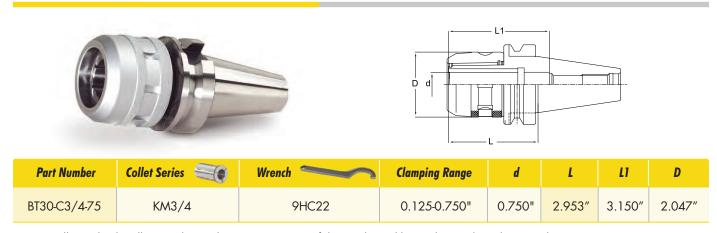
Note: Milling Chuck collets are located on pages 17-22 of the Lyndex-Nikken Advanced Product Catalog. Spanner wrench not included.
