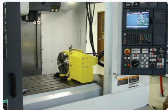
4th axis installation and interface on Mori Seiki NV5000
