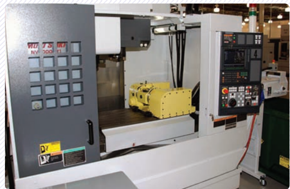
5th axis installation and interface on Mori Seiki Vertical Machining Center
