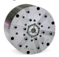
Large Diameter Air Chucks offer high accuracy and adjustable clamping force for machining large diameter precision and thin-walled workpieces. Large Diameter chucks are available in three jaw as well as two and six jaw configurations. Large Diameter models with extended jaw stroke, air ports on OD of chuck body for stationary applications, and other special configurations are quoted upon request.
