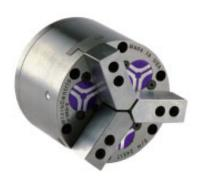
Long stroke air chucks feature extended jaw opening for load clearance or to clamp a range of diameters without changing top jaws. Long stroke chucks are available in rotating and stationary configurations. Their high accuracy makes them ideal for clamping headed workpieces for turning, grinding, or milling/drilling applications.
