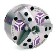
Rotating air chucks are ideal for precision turning and cylindrical grinding applications that require close concentricity, squareness, and parallelism tolerances. Variable clamping force enables clamping of thin-walled and other fragile parts with minimal distortion. All models, except the 3-50, feature a coolant or air passage through the center of the chuck.
