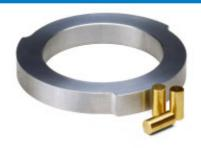
Loading rings are used to set the chuck in a clamping position when machining top jaws. CR loading rings provide easy adjustment of the loading position for OD holding applications. The LR loading rings are used for ID holding applications.
