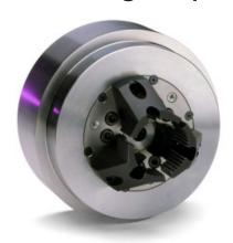
HST High Speed Air Chucks feature a titanium chuck body and are actuated by a patented external wedge design that maintains clamping force at high spindle speeds without counterweights. This revolutionary design minimizes the effects of centrifugal force resulting in consistent clamping force throughout the chuck's rpm range.
