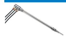
MicroCentric's patented NR50 air tube is used with HST/HS chucks. This air tube couples to a rotary air journal mounted in the ID HST/HS chucks. The NR50 is a three passage design for coolant through the spindle or automatic lubrication.
