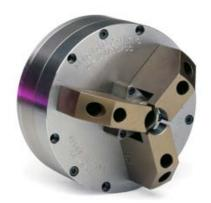
Sealed air chucks feature a stainless steel cover that seals the jaw slides. This design prevents contamination from grit and swarf and minimizes chuck maintenance for high volume production operations. Sealed air chucks are available in rotating and stationary configurations and are ideal for cylindrical grinding operations as well as machining abrasive materials such as powdered metal, ceramic, or carbide.
