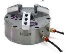
Stationary air chucks are ideal for milling, drilling, tapping, and other applications requiring a compact self-contained workholding fixture. Air is supplied directly into the side of the chuck body, and the chuck can be mounted directly to the machine table or pallet. Through holes are available on all models.
