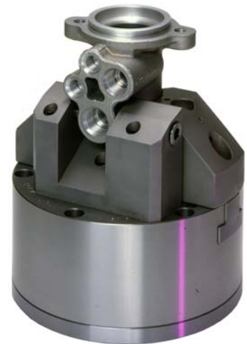
2 Jaw Air Chuck with special top jaws and part locator
