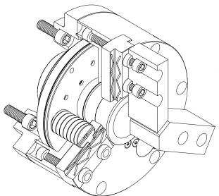
PPC chucks feature a patented open center design with separate actuators mounted to a piston connected to the draw tube adapter.
