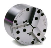
Long Stroke PPC chucks provide a larger jaw stroke for load clearance or to accommodate a range of clamping diameters without changing top jaws. PPC chucks can be actuated by a hydraulic or pneumatic cylinder, and can be adapted to any machine spindle or workhead configuration. PPC chucks include a spindle mounting plate and draw tube adapter.
