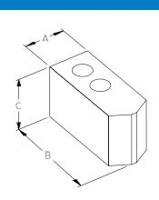
Blank QC Top Jaws are made from A-2 tool steel and feature finish machined tapered seats for accurate location. Blank QC jaws can be heat treated to a hardness up to Rc 62.
