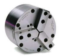
Standard series PPC chucks are designed for precision turning and cylindrical grinding applications required to hold close concentricity and squareness tolerances. PPC chucks can be actuated by a hydraulic or pneumatic cylinder, and can be adapted to any machine spindle or workhead configuration. PPC chucks include a spindle mounting plate and draw tube adapter.
