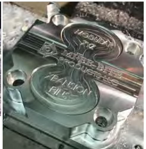
Op 2 including c'bore on same fixture
