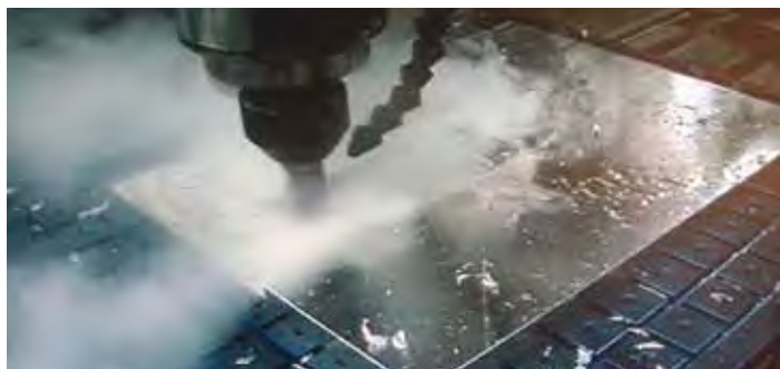
Application using Mitee-Grip™ with sacrificial top plate
