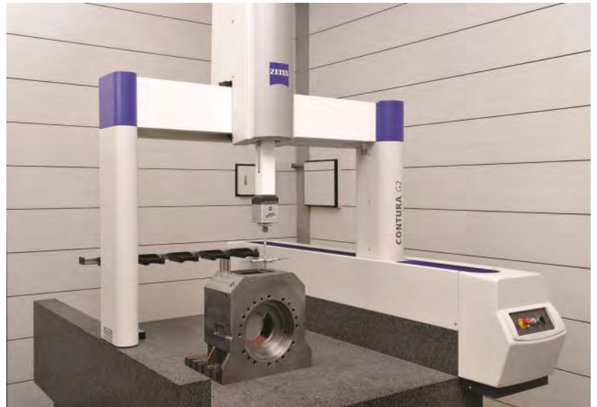
ZEISS CMM for components inspection
