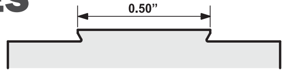
Raptor Interface=(4) C'Bores on a 3.800" B.C. for 1/2-13 or M12 SHCS with a 1.250" x .250 Boss
