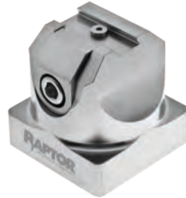
Raptor Interface=(4) C'Bores on a 3.800" B.C. for 1/2-13 or M12 SHCS with a 1.250" x .250 Boss
