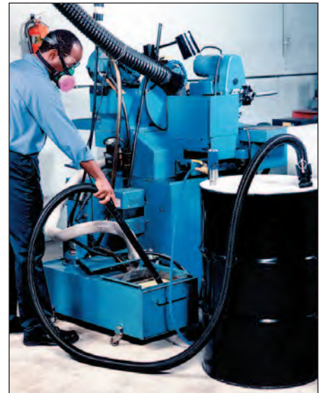
The Royal PneuVac pump filled this 55-gallon drum with coolant in less than two minutes.
