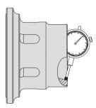
Much more accurate than S-type collet chucks and no time wasted boring jaws.
