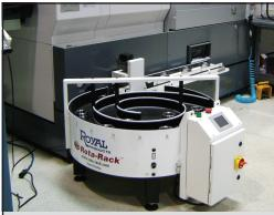
The Royal Rota-Rack® is an automatic accumulator that can be used with any bar-fed CNC lathe to safely collect finished parts, providing hours of highly profitable, unmanned production.
