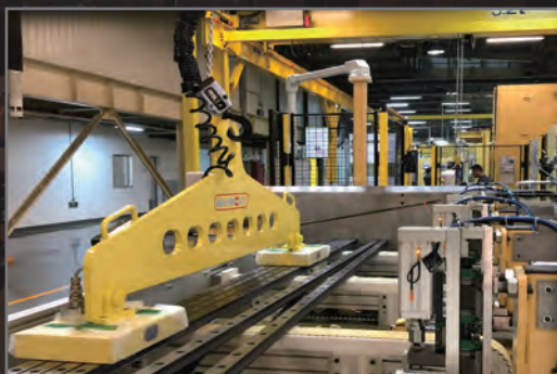
■ Helmholtz lifting magnets are BTH-1 and B30.20 compliant
