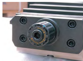
2. Rotate the adjustable knob to the required torque setting.
