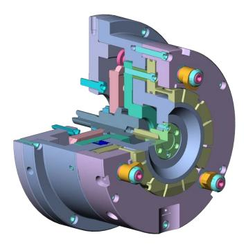
This chuck was built to hold a workpiece for the appliance industry. The internal collet is spring actuated, and the swing clamps are actuated by the machines drawbar.
