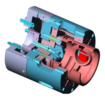
The workpiece is a piston for large heavy duty trucks. Gripping on the OD of the workpiece. The collet has inserts that can be changed for various piston OD's coolant is introduced thru the center to help flush out chips.
