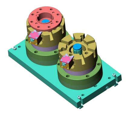
The workpiece is for the automotive industry. The collet grips on the ID of the part and radially locates externally on a cast boss.
