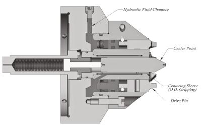
The convenience of a face driver with the accuracy of a hydraulic arbor
