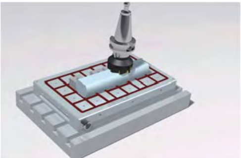
Example of machining the keyhole and surface of the round work piece
