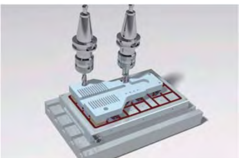
Example of machining with fixed pole extension blocks and turn pole extension blocks
