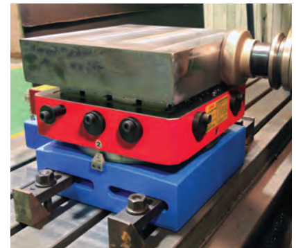
For workholding of ferrous materials only
