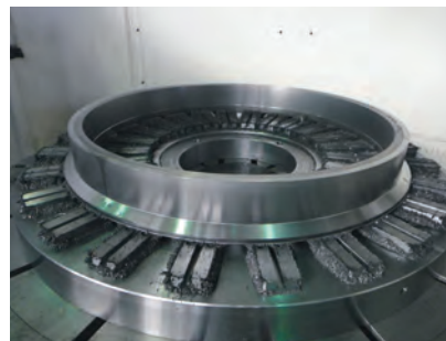
Even workholding - no part distortion
