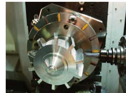
Off-axis rotation on horizontal mill
