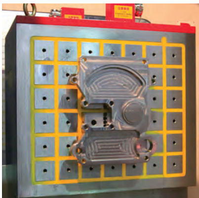
Complex part shapes - 5 sides machining
