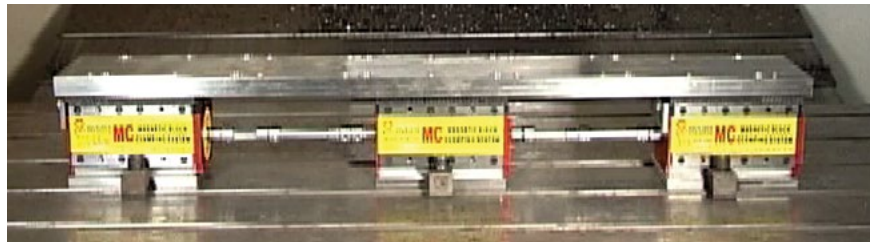
Switch-connect ECB vises to turn ON/OFF simultaneously
