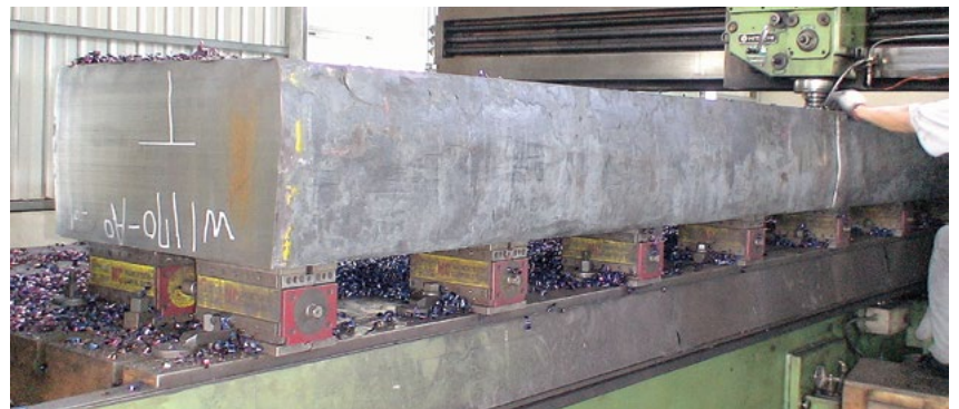
Even huge workpieces like this one are easily held and can be machined on 5-sides.
