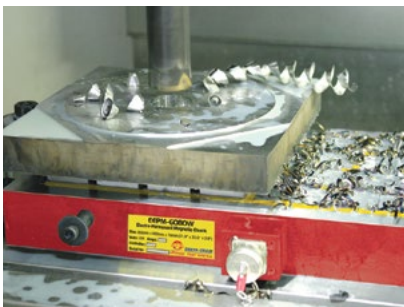
High holding power for heavy cutting
