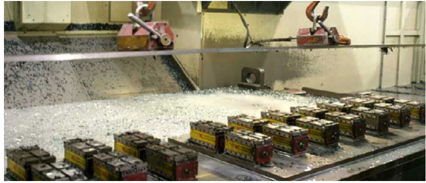
...or use multiple ECB vises positioned as needed to hold large parts.
