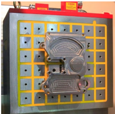
Complex part shapes - 5 sides machining
