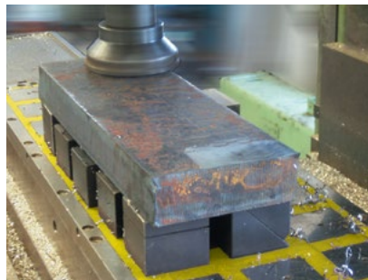
Use spring-loaded blocks for warped stock
