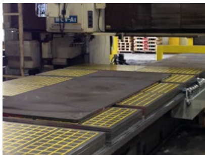
Custom solution for holding large flat plates
