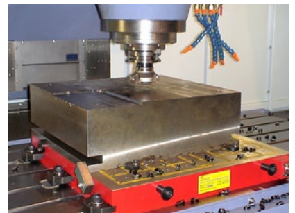
Face milling on workpiece with work-stops installed
